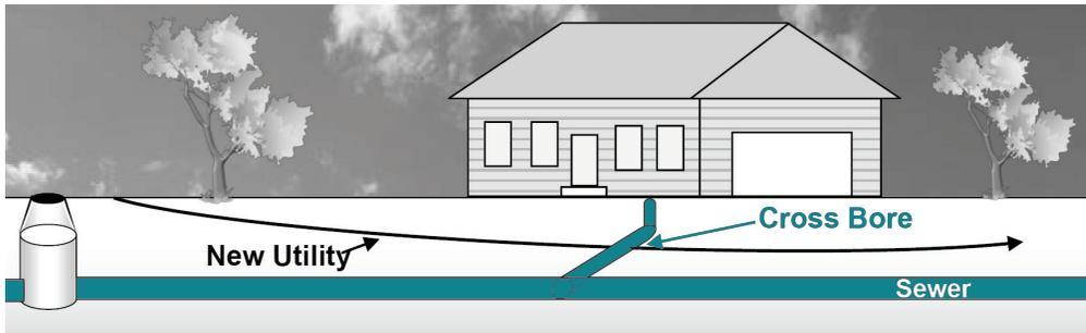
There is a possibility that our gas pipeline may cross through the sewer pipe on your property. This is called a cross bore and occurs when trenchless technology was used to install underground utility lines.
