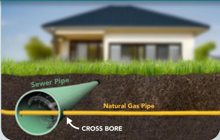
Plumbers and homeowners often use a rotating cutter to clear clogs in sewer lines. While this tool is good for clearing obstructions such as tree roots, these devices may also cut through a natural gas pipeline or other underground utilities that intersect the sewer line.
