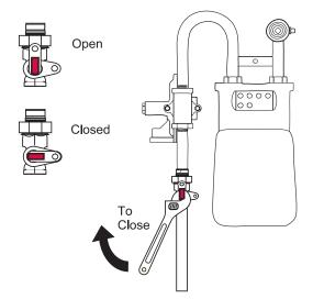
Use a long-handle wrench to turn the valve one-quarter turn so that the lever is crosswise to the pipe (see diagram).
